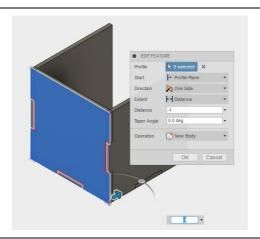
31. You are now ready to extrude the front face of the cube. Click Create > Extrude, then select the profiles to extrude. Distance is –t and Operation is New Body. Click OK.
